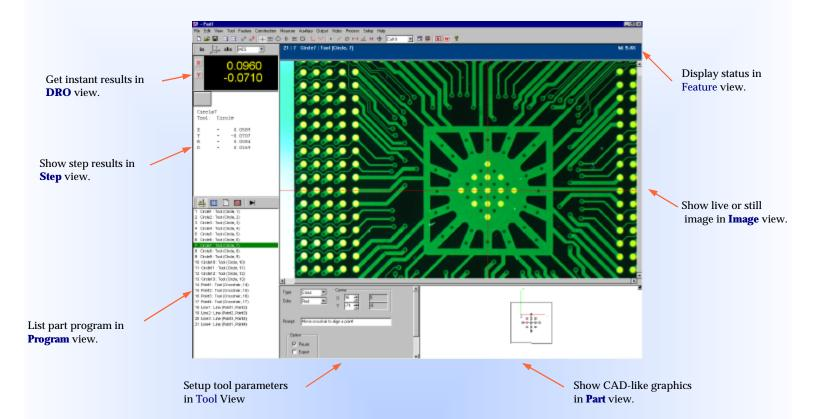
The DMP-2000 software is a PC-based field of view dimensional measurement & Imaging software that turns a conventional microscope into a powerful measurement system. The software uses the latest digital image processing technology to capture and analyze video images for dimensional measurement. It then compares the measurement to nominal values and tolerances to identify conditions of nonconformance. The DMP-2000 tolerance functions conform to ASME Y14.5M 1994.
