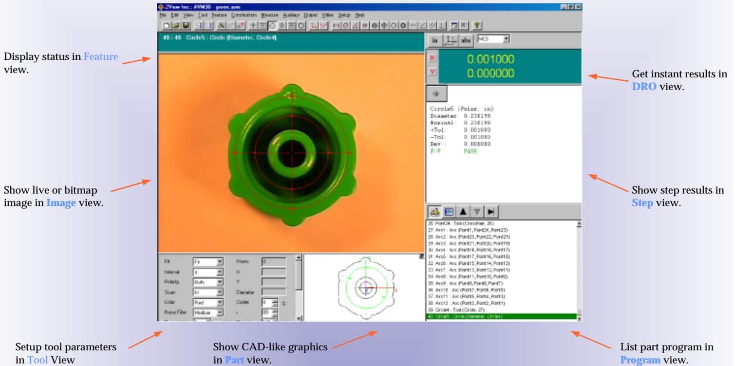
The AVM30 software from ZView is a PC-based field of view dimensional measurement software that turns a conventional microscope into a powerful measurement system. The software uses the latest digital image processing technology to capture and analyze video images for dimensional measurement. It then compares the measurement to nominal values and tolerances to identify conditions of non-conformance. The AVM30 tolerance functions conform to ASME Y14.5M 1994.
